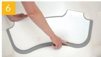
6 To ensure the rubber gasket lip is completely flat, run your finger around the front and rear of the gasket to check for a perfect seal.
